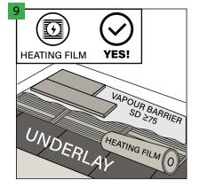
Installation on a heating foil is also allowed, provided that an appropriate underlay for the heating film and a vapor barrier foil SD ≥75 are used. The entire system consists of a vapor barrier foil laid directly on the substrate, then an appropriate underlay (min. 400 kPa, the recommended thickness of the underlay is 5 mm), a heating foil, a vapor barrier foil and the floor.
