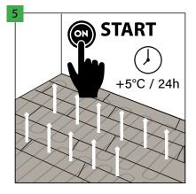
After laying the floor and waiting 24 hours, you can turn on the underfloor heating, remembering to gradually increase the temperature (5°C per day). ATTENTION! It should be remembered that the maximum temperature of the floor surface is 27°C.
