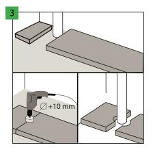
In the case of vertical pipes embedded in the substrate, leave free space around the pipes. Holes for the pipes must be drilled with a drill bit with a diameter that is bigger than the pipe diameter by 5 mm.
