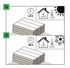
If the temperature is >5°C during transport, the acclimatization time in a room with a temperature of 18-30°C should be min. 24 hours (in the premises where they will be installed). However, in case of temperature <5°C during transport, acclimatization time in a room with a temperature of 18-30°C should be min. 48 hours.
