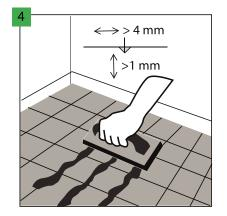
In the case of installation on the substrate covered with ceramic tiles, fill the tile joints with the gap wider than 4 mm and deeper than 1 mm with a durable compound for the filling of points, e.g. resin grout. Installation is allowed on tiles with grouts not wider than 5 mm and 1 mm deep without using levelling compound, provided the Multiprotec Hardlay or Vinclic Solid are used as underlay.
