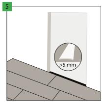
The application of the 5 mm expansion joint in the door opening between the rooms, which allows for the elimination of stresses, is recommended in the following cases: the irregular shape of the floor surface in the neighbouring rooms, the placement of heavy furniture in one of the rooms or the application of the underfloor heating only in one of the joined rooms. In the case of an area bigger than 200 m<sup>2</sup> or longer than 20 m, the expansion joint must be enlarged to 10 mm.
