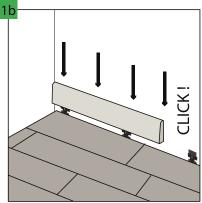
Expansion joints along the walls must be covered with a decorative strip, assembling it by means of glue or special clips. It is recommended to use the Arbiton strips dedicated to a given panel, which guarantee the excellent colour match and the coat resistant to scratching.
