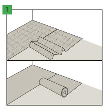
Lay the Arbiton, Ewifoam or Afirmax underlay perpendicularly to the direction in which panels are laid. The neighbouring ribbons of underlay must be fit tightly and joined by means of an overlap or Arbiton AluTape, without leaving any redundant space.
